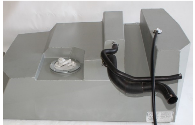
Photo 3: Fit hoses and pickup unit
