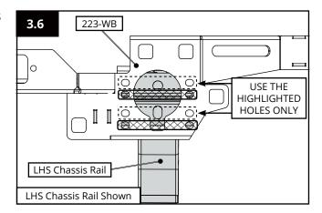
Reattach OE inner chassis rail support bracket between RHS chassis rail and 223-WB. Insert spacer between OE inner chassis rail and 223-WB, then insert hardware.
