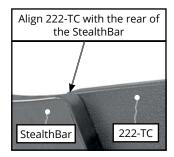
StealthBar x12 Stitch screws Backside of StealthBar
