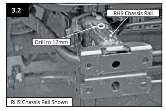
**Note:** Do not fully tighten any of the brackets until final alignment of the bar is finished.
