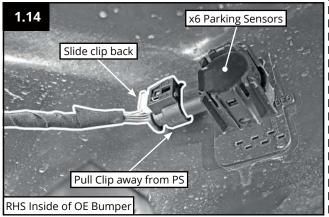
1.15 Disconnect the parking sensors from the bumper skin, take note of parking sensor orientation and location, retain for later use.
