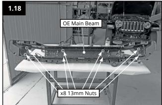
1.19 Remove OE Lower Tow Loop from main beam, retain for later use. Discard Main Beam.
