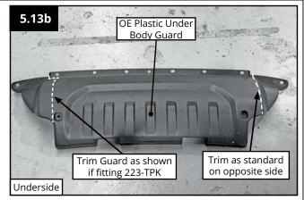
**Note:** To allow usability of a high lift jack, the area shown needs to be cut to allow the SAHLJ2 to fit into position. SAHLJ2 Sold separately.
