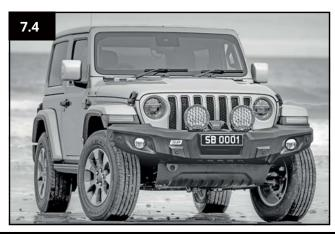
7.5 Finished StealthBar with replacement tow point, replacement steel skid plate and replacement fog lights.
