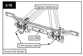
3.18b With all fasteners in place and bracket 223-WB centred between the chassis rails, tighten all to the appropriate torque.
