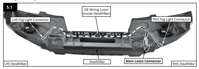
5.3 Feed the wiring loom inside of the StealthBar using an electrical snake. Feed loom through making sure the main connector is on the RHS as shown.
